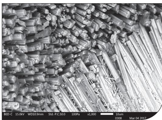
**Fig. 3.** SEM image of M/U2523.1 (romanechite) sample. Scale bar is 10  $\mu\text{m}$ .
