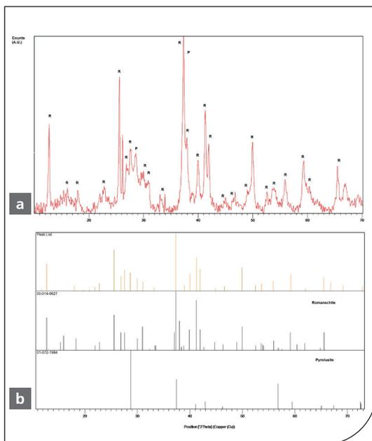
**Fig. 2.** XRD pattern (a) and peak list (b) of M/595 sample. Abbreviations: R, Romanechite, P, Pyrolusite.
